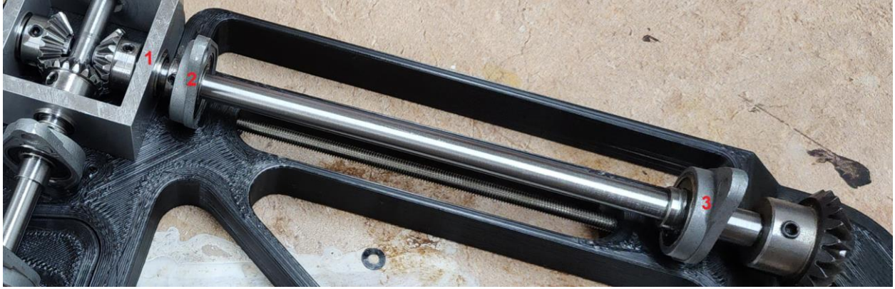
Figure 3.5 The three support bearings. Bearing number 2 was discarded in the final assembly
