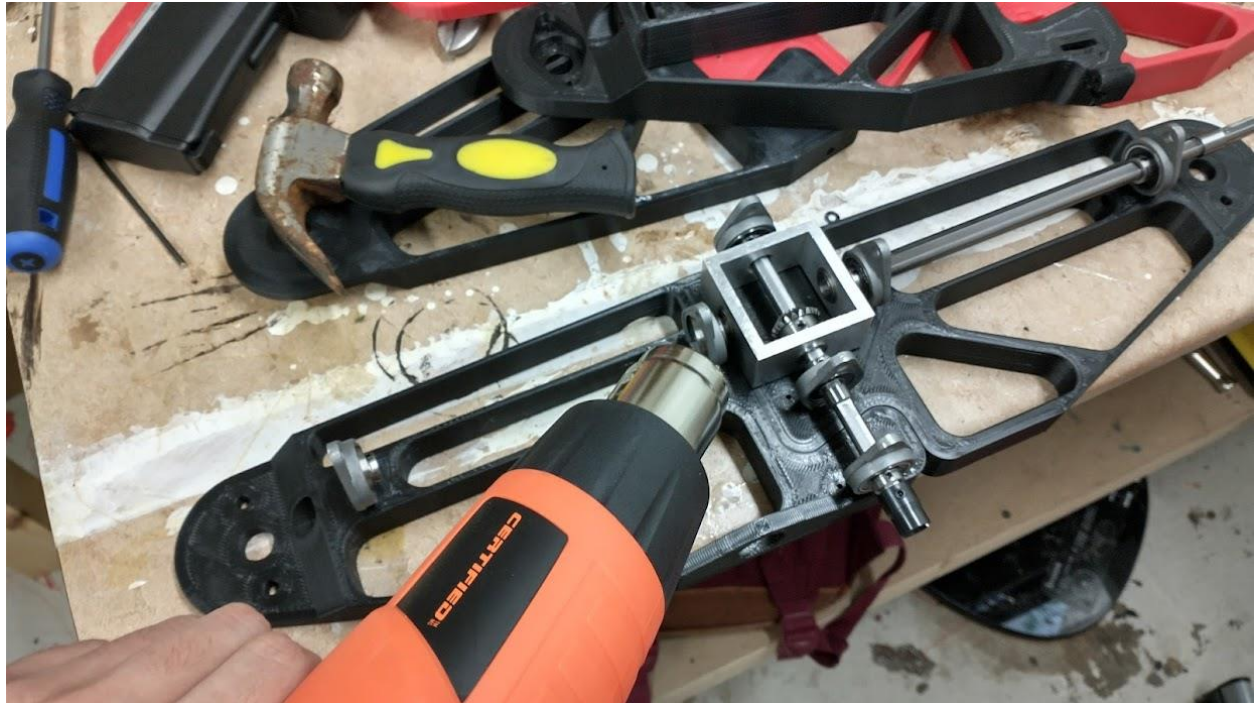
Figure 3.33 Heating up the pillow block bearings
