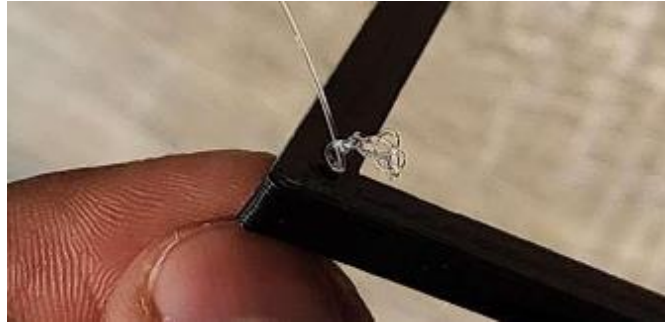
Figure 3.40 The wire passing through the spacer
